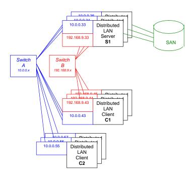
In the diagram there are two subnetworks: the blue subnetwork (10.0.0.x) and the red subnetwork (192.168.9.x). Servers such as S1 are connected to both the blue and red subnetworks, and can each provide up to 2 GByte/s of throughput to clients. (The three servers shown would thus provide an aggregate of 6 GByte/s.)
