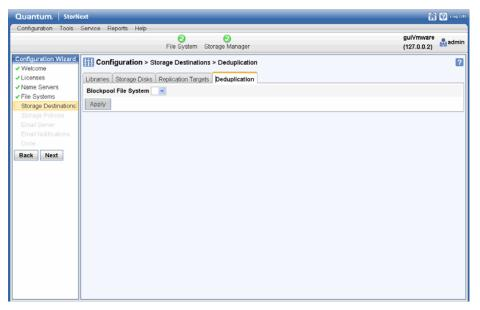
3 Click the **Deduplication** tab. This tab has only one field called **Blockpool Host File System**. At this field select from the dropdown list the file system to use for the blockpool. (This is the file system you created in the previous step.)
