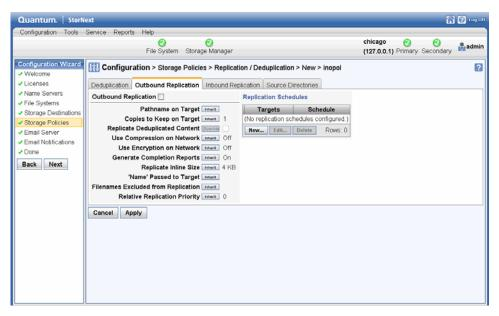
2 At the **Outbound Replication** field, enable outbound replication (going out from the source) by clicking the area to the right of the field so that **On** is displayed.
