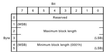
Figure 8-59 READ BLOCK LIMITS Data
