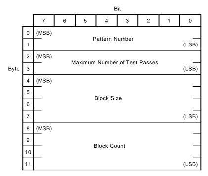
Figure 8-74 SEND DIAGNOSTIC Parameter List Format
