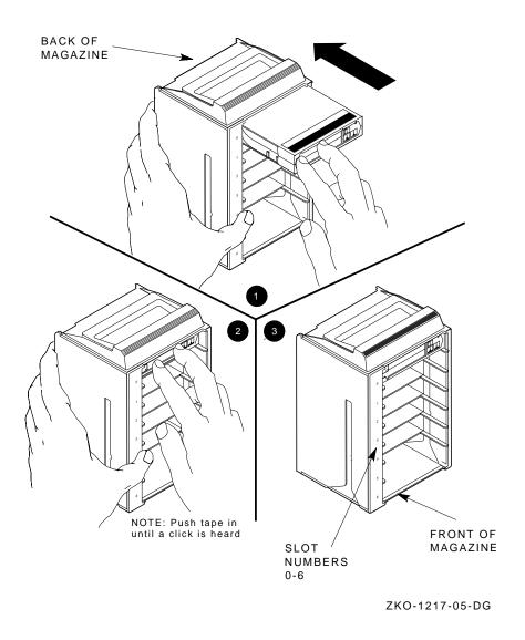
Figure 5-4 Inserting a Cartridge into the Magazine
