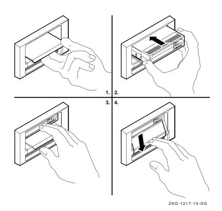
Figure 3-8 shows how to load a cartridge into the drive.
