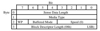
Figure 8-45 MODE SENSE (6) Data Header
