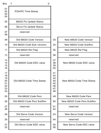
Figure D-6 Code Update (CUP) LOG Packet Layou
