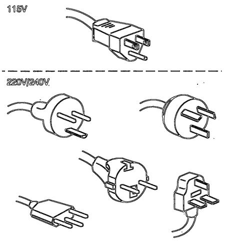
Figure A-1 shows the different AC power cord plug configurations for 115V and 220V/240V usage.
