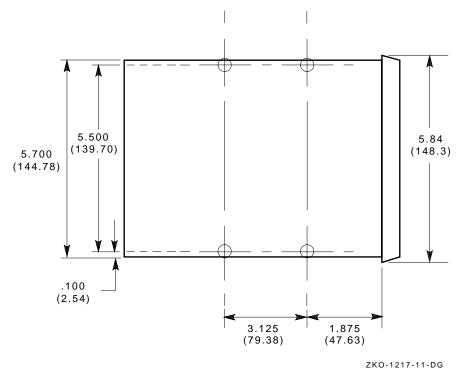
Figure A-2 shows the mounting holes and dimensions in a top view of the DLT2000 drive.
