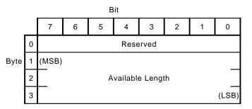
Figure 8-62 READ BUFFER Data Head
