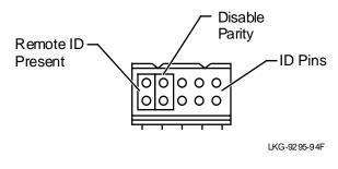
Figure 3-2 shows what the pins on the SCSI ID connector represent.
