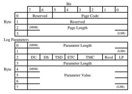
Figure 8-15 Read/Write Error Log Select Page Format
