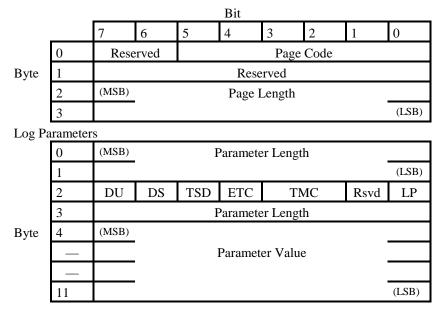
Figure 8-21 Read/Write Error Log SENSE Page Format
