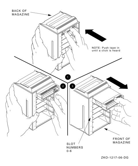
Figure 5-5 Removing a Cartridge from the Front of the Magazine
