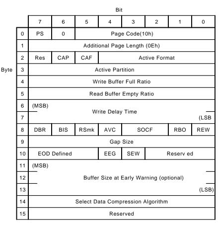
Figure 8-51 Device Configuration Page Format
