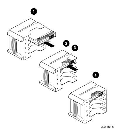
Figure 4-8 Inserting a Cartridge into the Magazine
