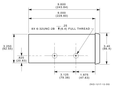
Figure A-3 shows the mounting holes and dimensions in a side view of the DLT2000 drive.
