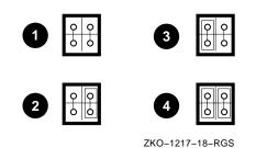
Figure 7-2 Jumper Settings for TRM PWR/TRM ENB Connector
