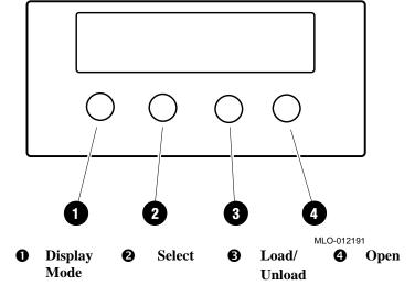
Figure 4-5 Mini-Library Operator Control Panel
