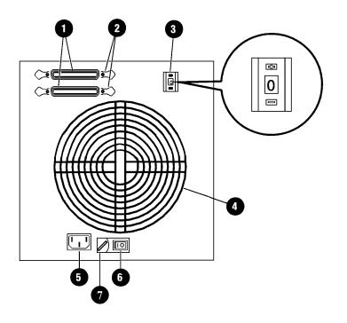
Figure 5-1 shows the location of the SCSI ID pushbutton switch.
