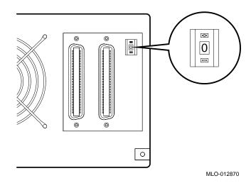
Figure 2-2 Changing the SCSI ID via the Pushbutton Switch
