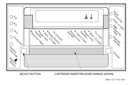
Figure 2-1 Drive Front Panel
