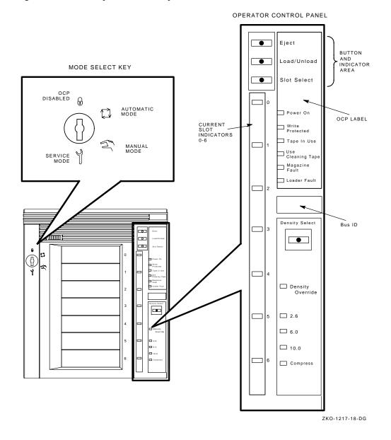
Figure 5-2 shows the operator's control panel.
