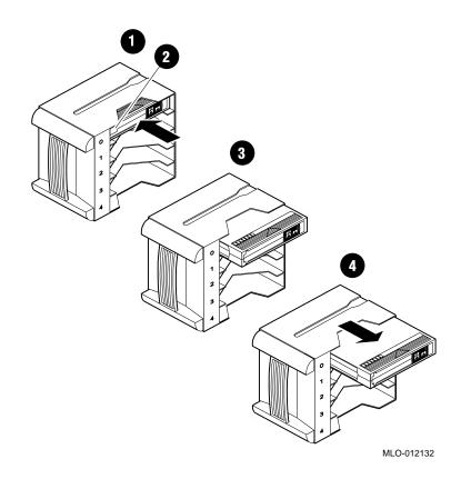
Figure 4-9 Removing a Cartridge from the Magazine
