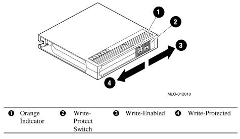
Figure 4-6 Write-Protect Switch on a Cartridge
