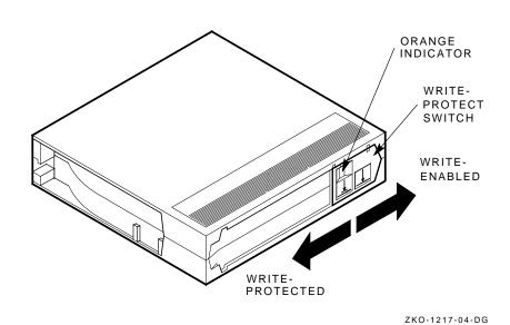
Figure 5-3 Write-Protect Switch on a Cartridge
