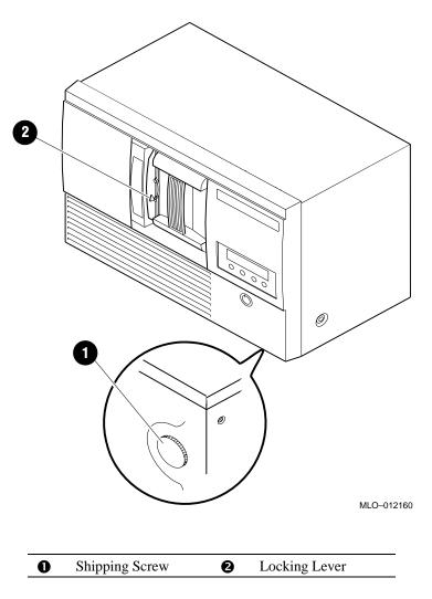
Figure 4-1 Loosening the Shipping Screw Under the Mini-Library
