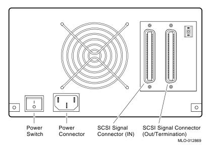
Figure 2-3 Rear Panel Components
