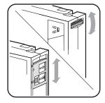
Write Protection Switch Move the switch. It should be able to snap into write-protected mode and write-enabled mode.
