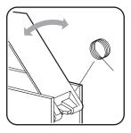
**Cartridge Door** Ensure the door is movable and that the spring is present.
