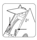
Toed-In Buckle Buckle ends clearly extend past edge of reel.
