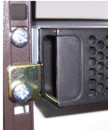
Figure 7. Fasten the front of the FastStor 1 to the rack.
