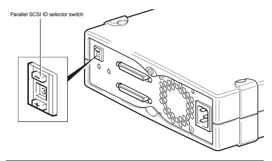
**Note:** Parallel SCSI controllers and host adapters generally use ID 7. In some systems, the boot drive uses ID 0 or ID 1. Avoid configuring the LTO-3 (Model B) Half-Height Tape Drive to these SCSI IDs.
