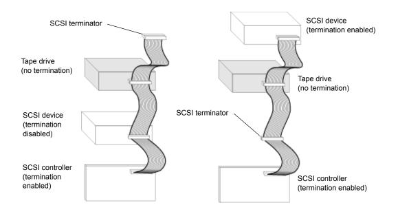
**Note:** The internal parallel SCSI LTO-3 (Model B) Half-Height Tape Drive does not provide SCSI termination. The last device at the end of the parallel SCSI bus chain must have a SCSI bus terminator.
