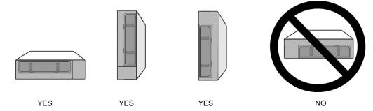
Mount the internal drive in a 5.25-inch, half-height drive bay as follows:
