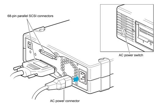
Figure 10 Tabletop SAS Drive Interface and AC Power Connectors
