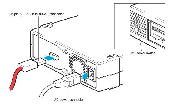
Connect the interface and AC power cables to the tabletop drive as follows:
