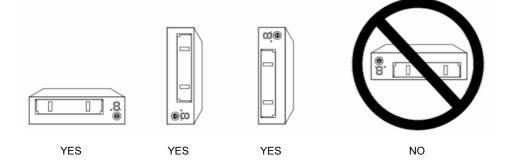
Mount the internal drive in a 5.25-inch, half-height drive bay as follows:
