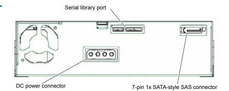
Connect the interface and DC power cables to the internal drive as follows:
