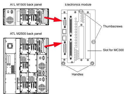
Figure 1 Removing the Electronics Module
