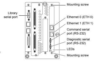
Figure 3 MC300 PMC Ports and Indicators
