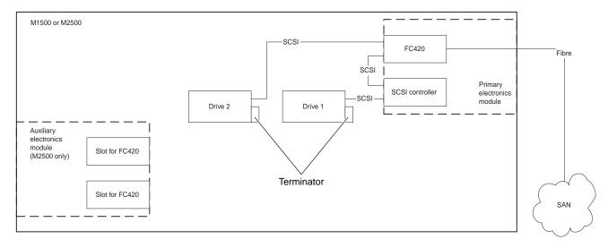
In a two-drive library, the second drive (drive 2) should be connected to the available FC420 port, creating a second SCSI bus. This utilizes the FC420 bridge fully and maximizes the communication bandwidth available to each tape drive.
