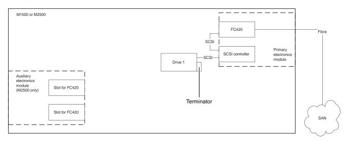
In a one-drive configuration (as shown in <u>figure 2</u>), a SCSI daisy chain is established from one of the SCSI ports on the FC420 bridge to the SCSI controller and then to drive 1, where the daisy chain is terminated. The SCSI controller is included in the chain to pass SCSI commands to the robot.
