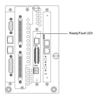
If there is an error, the Ready/Fault LED blinks in the following pattern:
