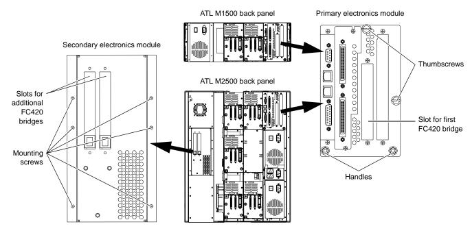
Figure 1 Removing the Primary and Secondary Electronics Modules
