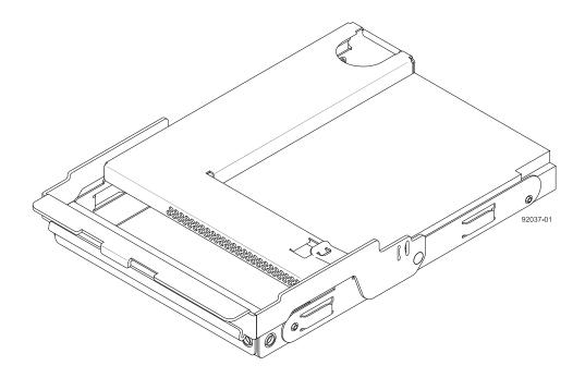
4. Push the drive drawer all the way back into the controller-drive tray, and close the drive drawer levers on each side of the drive drawer.
