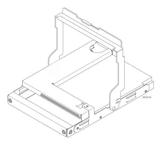
c. Lift the drive from the drive drawer by using the drive handle, and put the drive on a flat, static-free surface. If you are removing multiple drives, label each drive with the tray number, the drive drawer number, and the slot number. Then, if the fault is with the drive drawer and not the drive, the drive can be reused.
