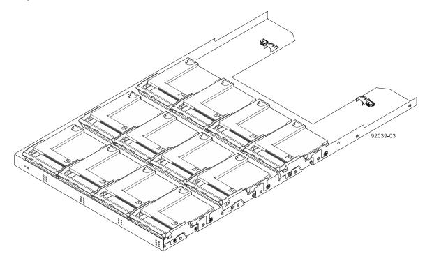
9. Remove the failed drive from the drive drawer by referring to "LEDs on the Drive -- Top View" (Figure 3) to determine which drive has failed. To remove a drive, perform these steps:
