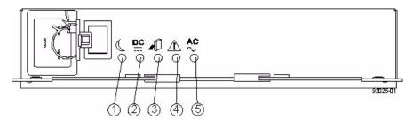
Figure 2 LEDs on a Power Canister
