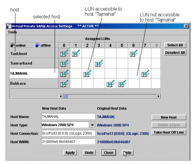
Figure 12 Scalar Firewall Manager access settings dialog box
