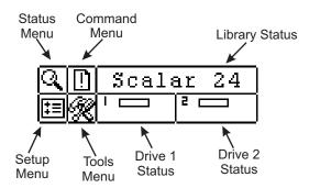
Refer to the Operation section of the Scalar 24 *Installation and Operation Guide* for complete descriptions of special symbols and messages that can be displayed on the Operator Panel.
