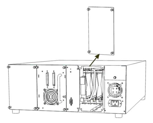
3 Slide the SNC into position until it mates with the connector then tighten the thumbscrews.
