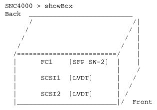
SFP SW-2 == Small Form Factor Plugable Short Wave Two GigaBit Optical LVDT = SCSI Low Voltage Differential - Terminated
