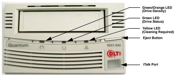
On the SDLT 600 tape drive, the leftmost LED is dual color (green/ orange). This LED is the Density Indicator. When you insert a Super DLT tape II data cartridge, this LED illuminates green. When the tape drive detects a backward read compatible (BRC) data cartridge, this LED illuminates orange. (For BRC details, see <u>Backward Read Compatibility</u> (<u>BRC) Transfer Rates</u> on page 34.)
