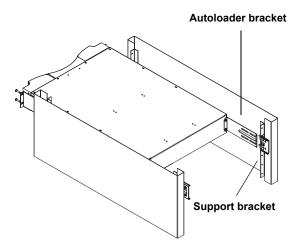
**5** While the other installer holds the front end of the autoloader, secure the front end of the autoloader to the rack using four rack screws (two per tab) as shown in <u>figure 6</u>. Tighten the screws just enough to secure the autoloader to the front rails.
