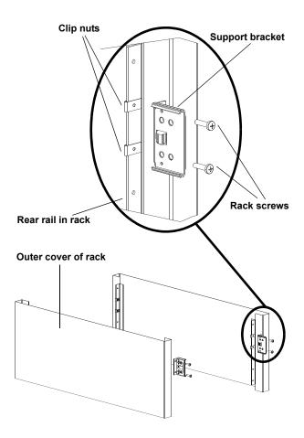
**4** With the help of a second installer, insert the autoloader into the rack so that the autoloader brackets slide into corresponding support brackets on the rear rails and the tabs at the front of the autoloader align flush with the clip nuts on the front rails (see <u>figure 5</u>).
